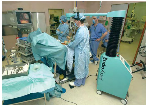
The EndoAssistant manipulates a laparoscopic camera at the command of the surgeon
