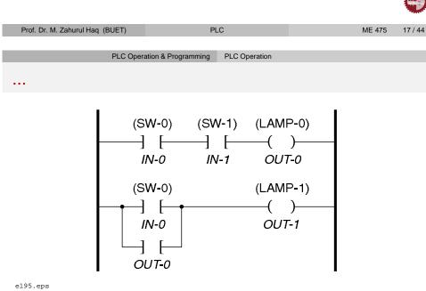
The ladder diagram (LD) has two rungs. The top rung will light Lamp-0 & if both SW-0 and SW-1 are closed. The bottom rung will light Lamp-1 if either SW-0 or OUT-0 are closed.
