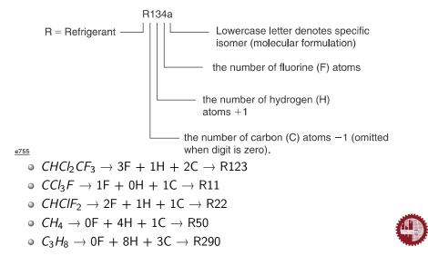
Numbering of Refrigerants: Halocarbon/Hydrocarbon
