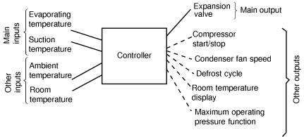
Electronic expansion devices are now widely used on automatic system in an integrated control circuit.
