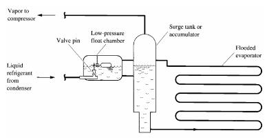
It controls the liquid refrigerant feed to maintain a constant liquid level in the evaporator. As the liquid level in the evaporator drops, the float ball, moves downward and opens the float valve wider so that more refrigerants feed to the evaporator.
