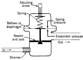
AXV's maintain a constant pressure in the evaporator by flooding more or less of the evaporator surface in response to the refrigeration load. It close off tightly when the compressor cycles off and remains closed until the compressor cycle is on.
