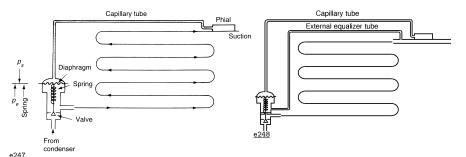
TXV's are the most widely used refrigerant flow control device. Operation is based on maintaining a constant degree of suction superheat at the evaporator outlet. In case of possible large pressure drop in evaporator, equalizing connectors are often used.
