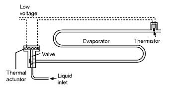
Signal from a suitable thermistor placed at the evaporator outlet will vary, depending on whether it senses dry refrigerant gas or liquid traces. It can be used to control the current through a thermal element to modulate in expansion valve.
