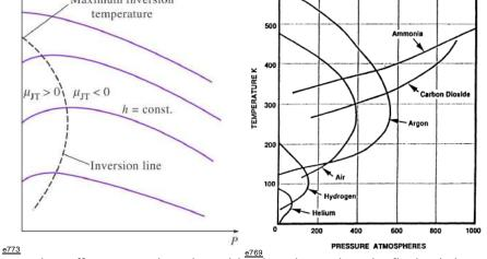
A cooling effect cannot be achieved by throttling unless the fluid is below its **maximum inversion temperature**. For hydrogen its value is -68°C and hydrogen must be cooled below this temperature if further cooling to be achieved.
