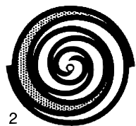
2 The pocket is sealed off, compression starts
