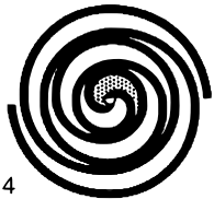
4 As the pocket reaches the centre, the discharge port is uncovered
