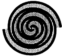
5 During the process all six pockets are in various stages of compression
