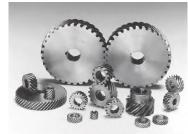
Helical gears are parallel-axis gears with teeth cut on helix that wraps around cylinder. These have greater load-carrying capacity than spur gears of the same size.
